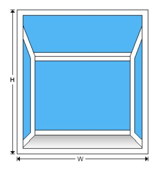
Window measurements needed: Separate width and height measurements in inches, rounded up to the next inch. Measure from side to side for width and top to bottom for height. (See illustration)
