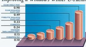
The U-Factor (also referred to as U-Value) is a number that represents the rate of heat flow through a glazing system. The lower the U-Factor, the greater a window's resistance to heat flow, and the better its insulating value. This performance is critical to those homeowners who may experience increased
