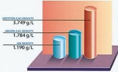
Insulated glass units were initially filled with air or dry nitrogen. It was later discovered that a dense, slow moving gas would help to minimize the convection currents within the space, thereby reducing conduction and the transfer of heat. These intersections are colorless and safe passes.
