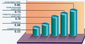
The solar heat gain coefficient (SHGC) is a number that represents the fraction of solar radiation admitted through a window, both transmitted and absorbed, and subsequently released inward. The lower a window's solar heat gain coefficient, the less solar heat it transmits, which therefore leads
