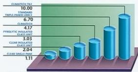
An R-Value is a measure of the resistance of a glazing material or fenestration product to heat conduction. It is the inverse of a U-Factor (R=1/U) and is expressed in terms of hr-sq ft-
